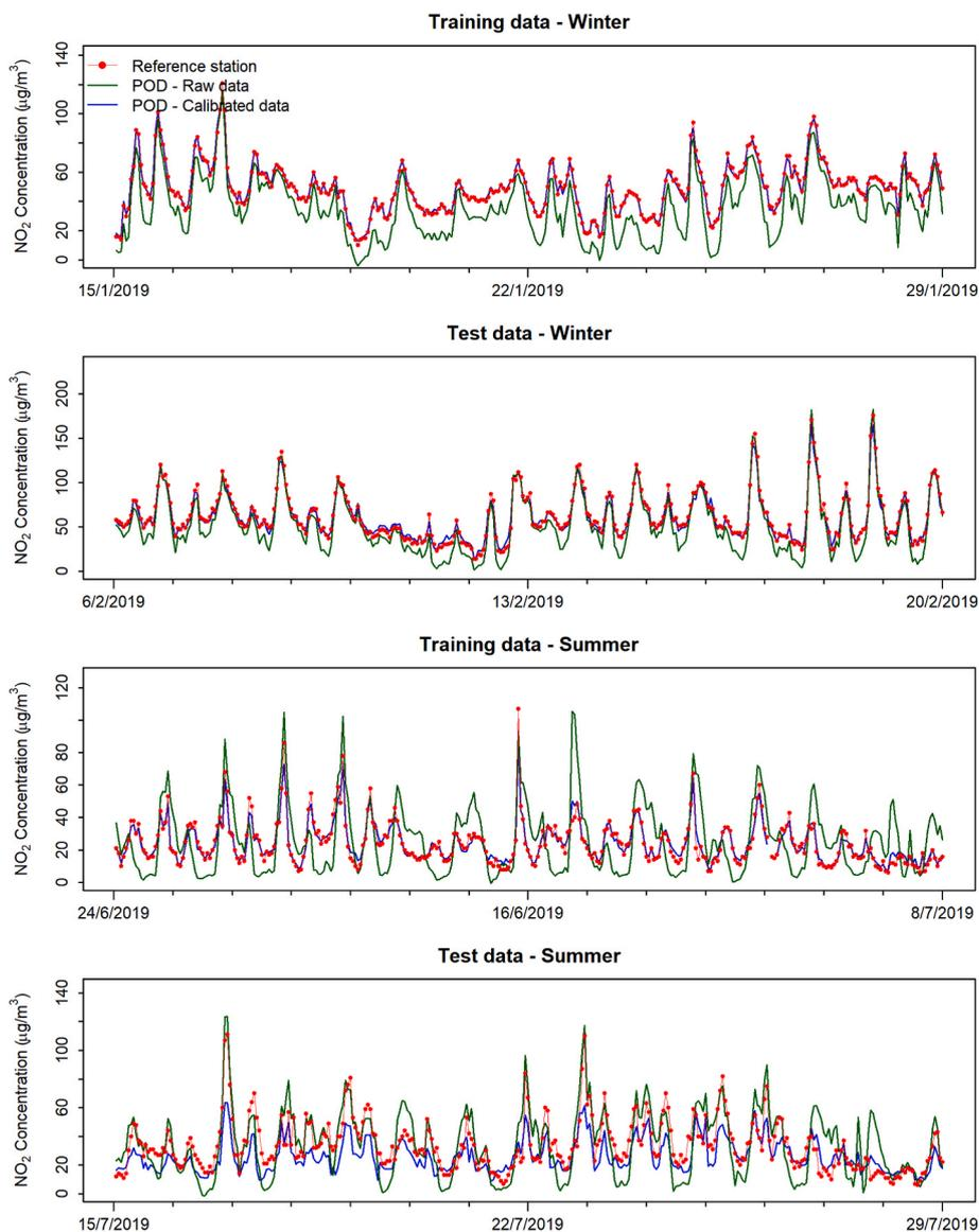
Fig. 7. Examples of comparison of NO<sub>2</sub> reference measurements with POD raw and calibrated data. Training data were collected at the urban traffic station in Parma (Period 4) while the testing data refers to the urban traffic station in Modena (Period 5).
