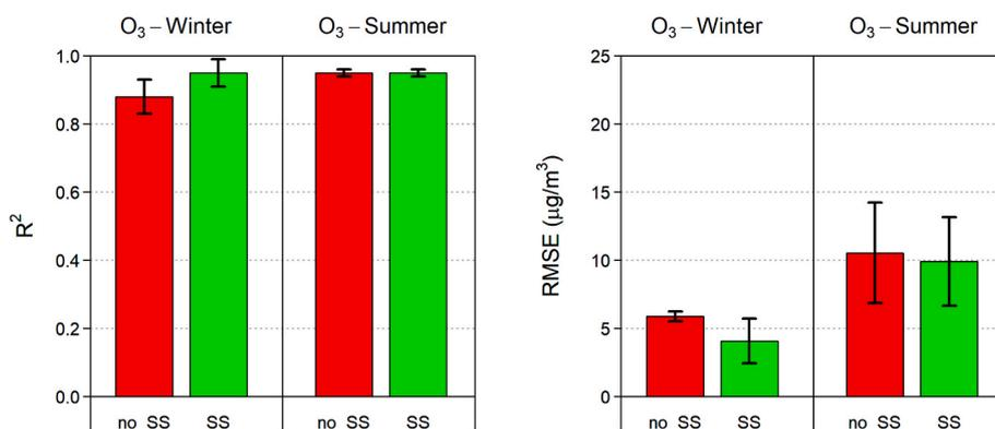
Fig. 5. Performance metrics ( $R^2$ , left panel; RMSE, right panel) for O<sub>3</sub> sensor tests. Mean and standard deviation of individual  $R^2$  and RMSE tests are shown.
