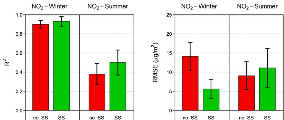
Fig. 8. Performance metrics (R<sup>2</sup>, left panel; RMSE, right panel) for NO<sub>2</sub> sensor tests. Mean and standard deviation of individual R<sup>2</sup> and RMSE tests are shown.
