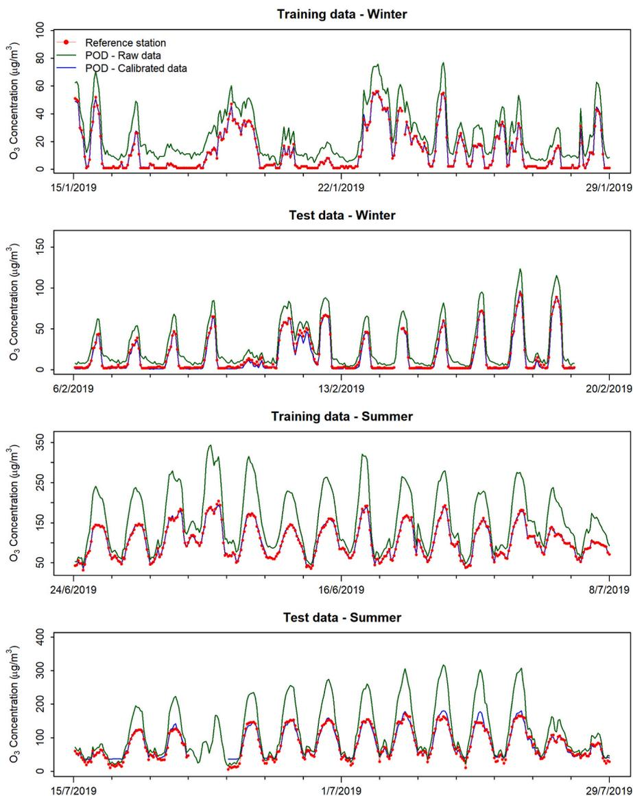
Fig. 4. Examples of comparison of O<sub>3</sub> reference measurements with POD raw and calibrated data. Training data were collected at the urban background station in Parma (Period 2) while the testing data refers to the urban background station in Modena (Period 3)..
