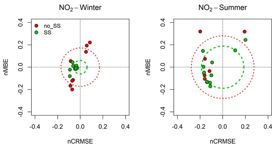
Fig. 9. Target diagrams for NO<sub>2</sub> for all testing periods grouped for season, and no\_SS and SS tests.
