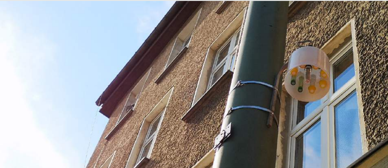
Figure 13: Passive sampler for measuring NO 2 at Brückenstraße, Berlin Mitte, Germany
