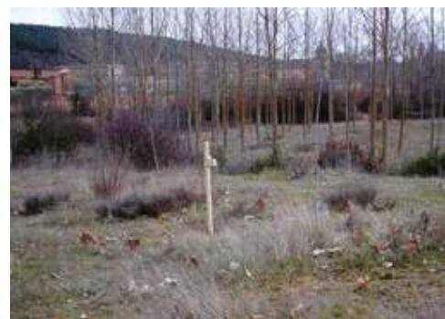
Outdoor radon detector placed 1 m above ground, Palencia province, Spain. Source: José-Luis Gutiérrez Villanueva.
