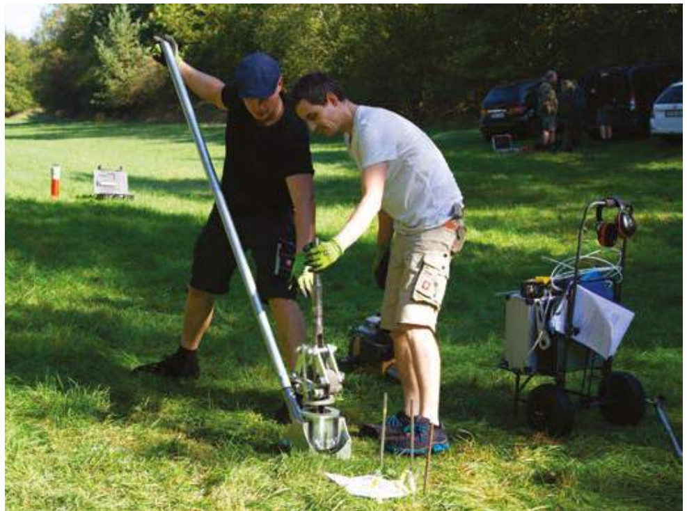
Soil-gas sampling drill, RIM 2018 exercise, Cetyne, Czech Republic. Source: Tore Tollefsen.
