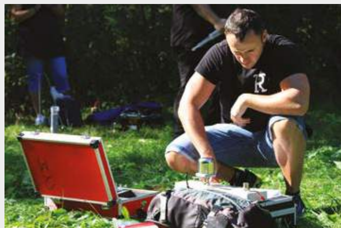
Field measurements of radon in soil gas, RIM 2018 exercise, Cetyne, Czech Republic. Source: Tore Tollefsen.
