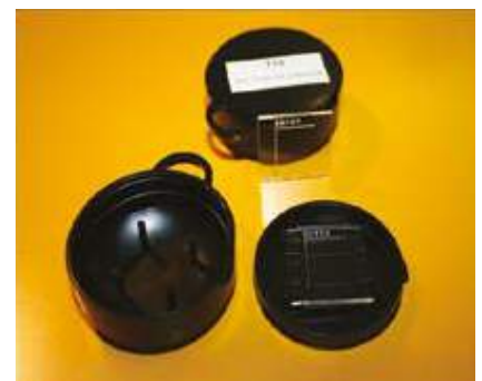
CR-39 track-etch passive radon detector. Source: EANR, EC-JRC, 2019.
