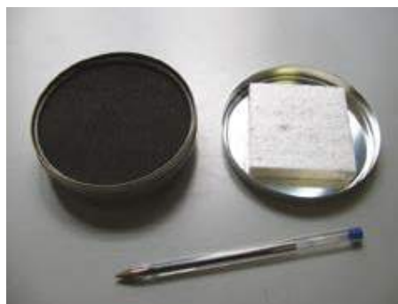
Charcoal canister used to measure indoor radon concentration. Source: Peter Bossev.
