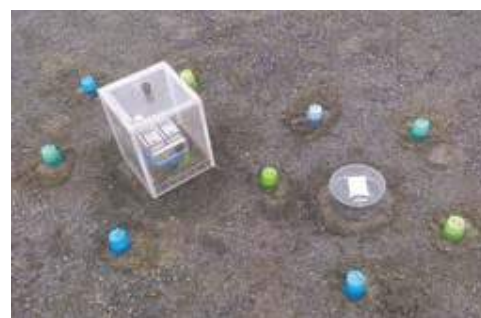
Radon exhalation rate measurements, Ciudad Rodrigo, Spain. Accumulation method using active monitors and charcoal cartridges (inside the plastic glass). Source: Luis S. Quindós.
