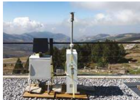
••• High-volume air sampler located at 2550m in Sierra Nevada, Spain, in the framework of the FRESA Project (ICGL2015-70741-R). Source: FRESA Project.
