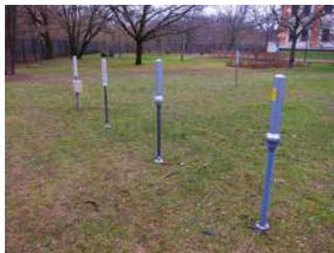
Test probes at the BFS premises in Berlin, showing antennas in various stages of development. Each can be equipped with a pair of Geiger-Muller counters, one for low and one for high dose rate. Source: Peter Bossew.
